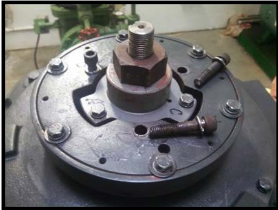
Sheared machine bolts on ratchet brake assembly on Matt Williams well motor.
