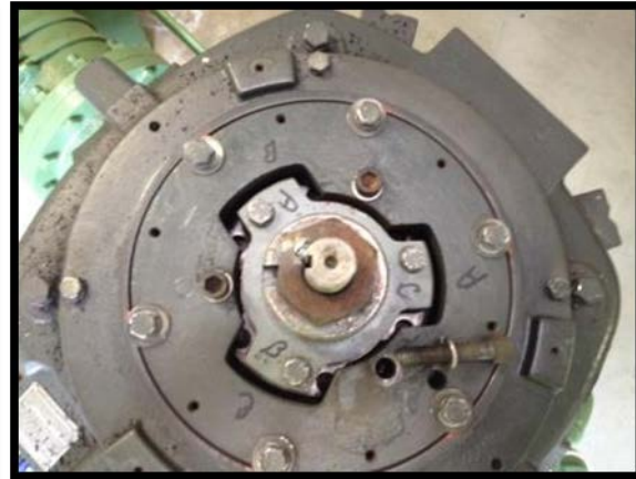
Sheared machine bolts on ratchet brake assembly on Matt Williams well motor.
