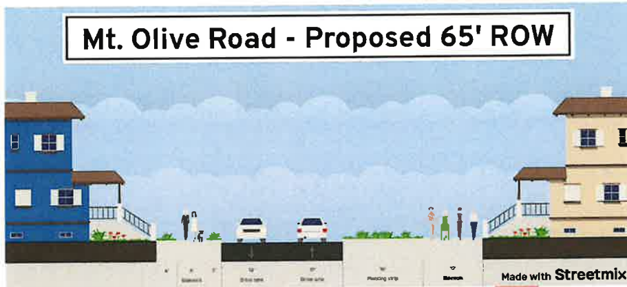
Figure 12: Mt. Olive Road Concept Typical Section with 5' Sidewalk and 12' SUP (65' ROW)
