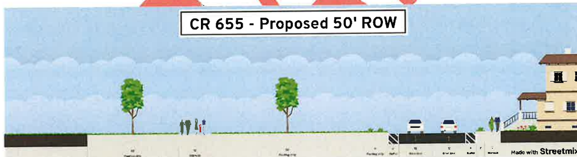
Figure 11: C.R. 655 Concept Typical Section with 5' Sidewalk (50' ROW).
