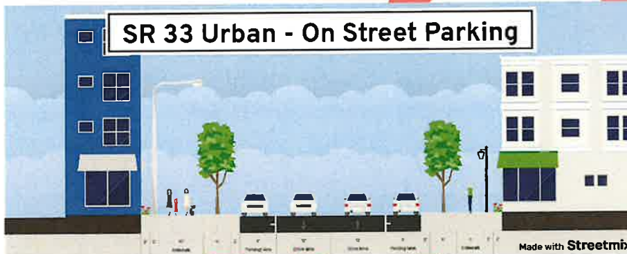
Figure 9: S.R. 33 Concept Typical Section with 10' Shared Use Path and Parking (80' ROW)
