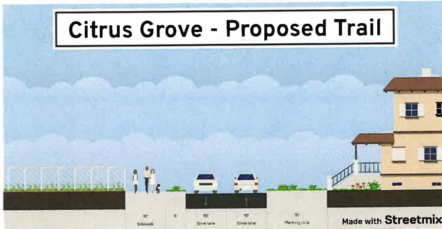
Figure 14: Citrus Grove Boulevard Concept Typical Section with 10' SUP (50' ROW)
