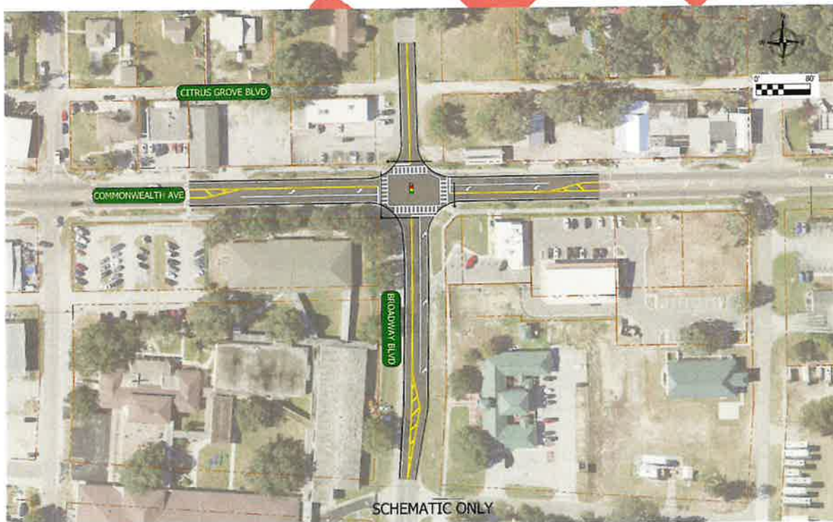
Figure 7: Signalized Intersection Concept at S.R. 33 and S.R. 559
