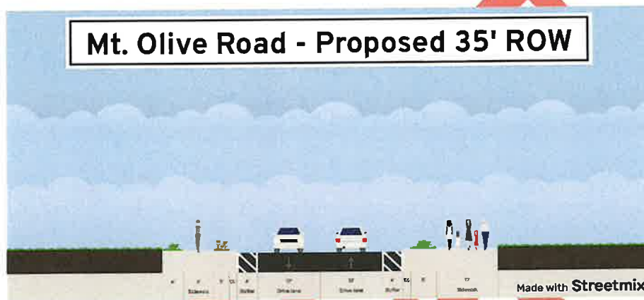
Figure 13: Mt. Olive Road Concept Typical Section with 5' Sidewalk and 12' SUP (35' ROW)
