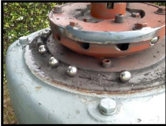
Top brake and ratchet gear came apart on 75hp motor at the Jacob WTP.
