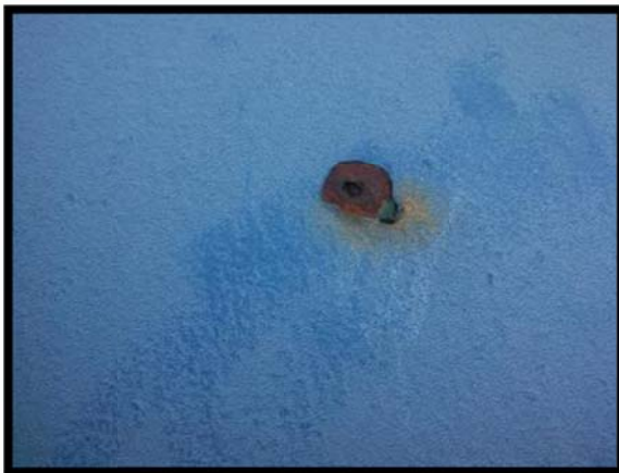
Hole found in the Matt Williams Hydrotank.
